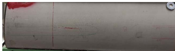
Figure 5: Front view of the sample used in the lab experiment. The vertical red line on the left side indicates a line defect beneath the surface.
