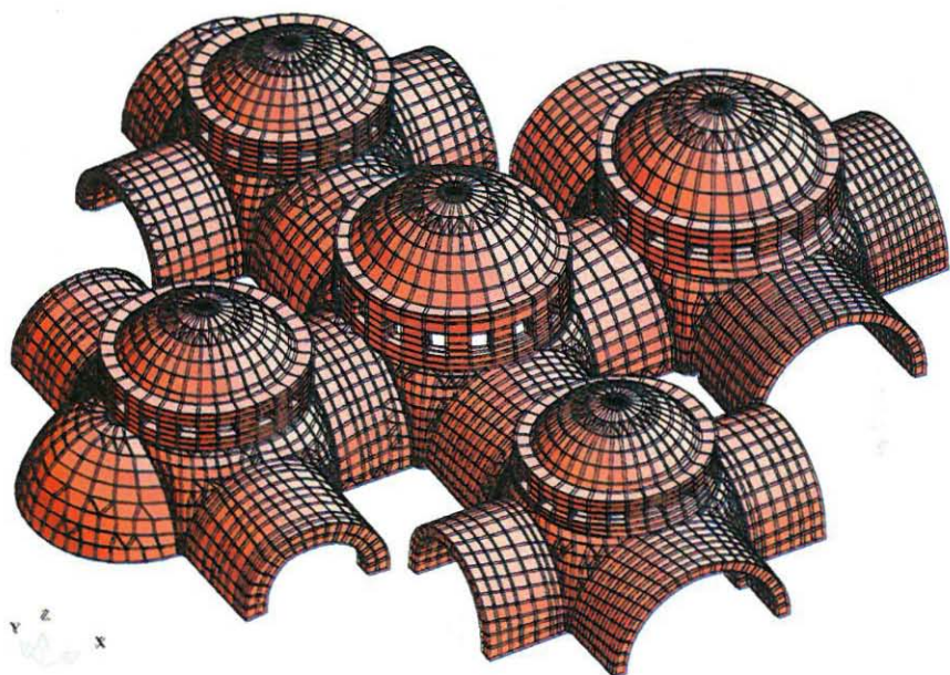
Figure 13. Finite Element mesh for the full 3D analysis of the 5 domes.
