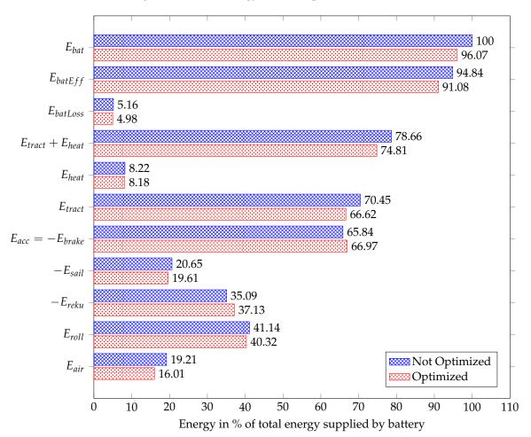
**Figure 6.** Comparison of the energy components for the recorded drive unoptimized and optimized. All values are expressed as % of  $E_{bat}$  of the unoptimized drive.
