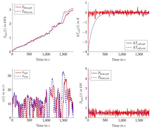
**Figure 7.** Comparison of optimized and unoptimized time series of the variables v(t) and  $P_{heat}(t)$ , as well as the components of the objective function  $E_{bat}(t)$  and  $\Delta T_{cab}(t)$ .
