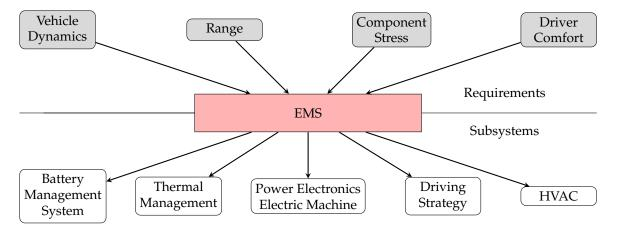
**Figure 1.** Example for the requirements and the subsystem managed by an energy management system (EMS) in a battery electric vehicle (BEV).
