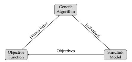
Figure 4. Interaction between the GA used for the optimization and the Simulink model.
