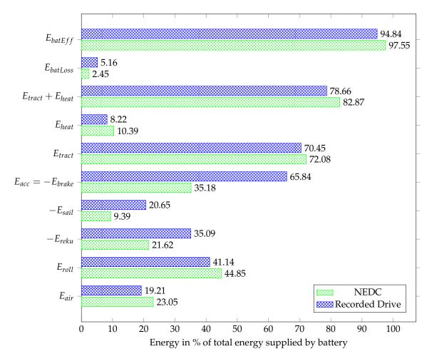
**Figure 5.** Comparison of the energy components for the recorded drive and the NEDC. All values are expressed as % of  $E_{bat}$  of the respective driving cycle.
