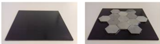
Figure 1. CFRP control plate (left) and CFRP plate with bounded ceramic hexagons on top (right).
