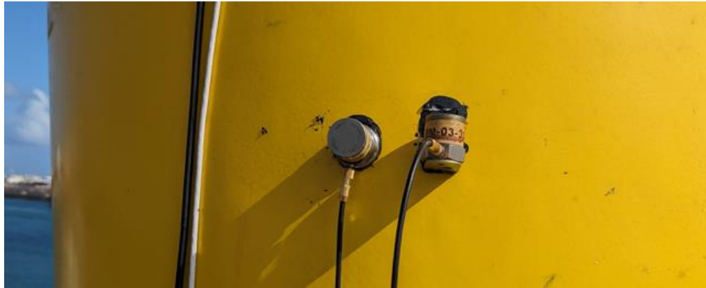
Figure 29 Unidirectional accelerometers installed at the FRP tower.
