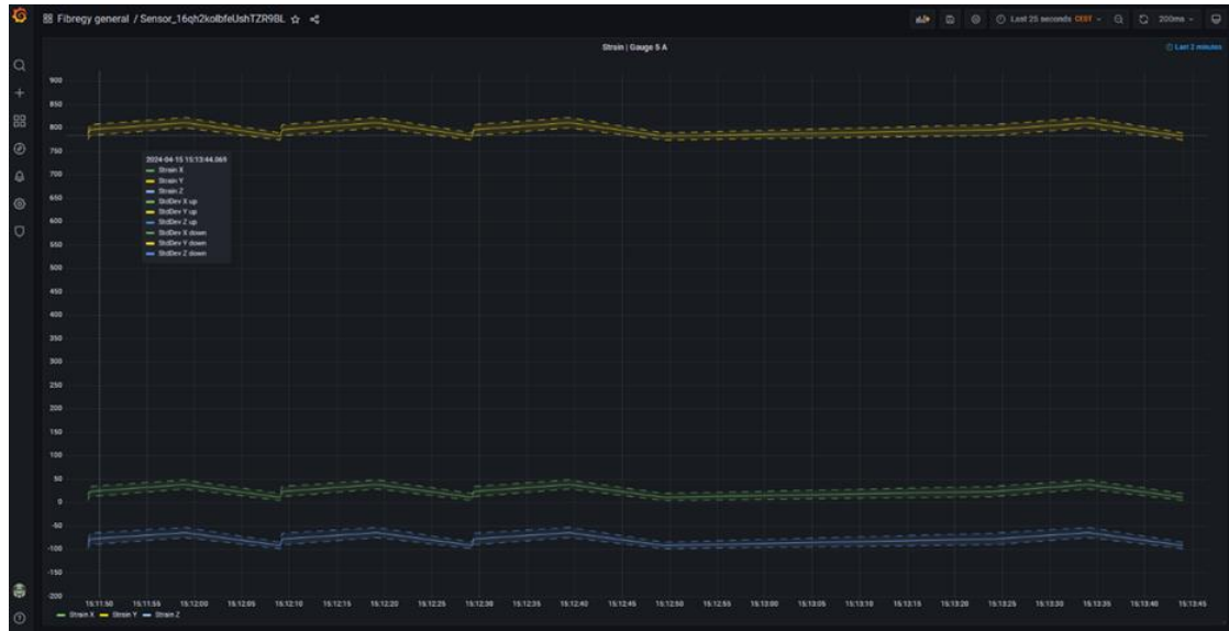
Figure 80 Processed data from sensor in the digital twin platform.
