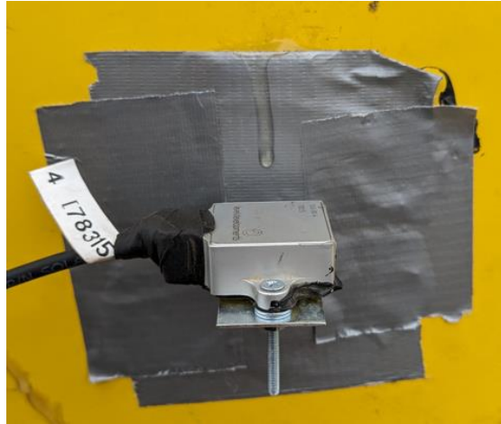
Figure 31 Instilled inclinometer at the FRP tower-
