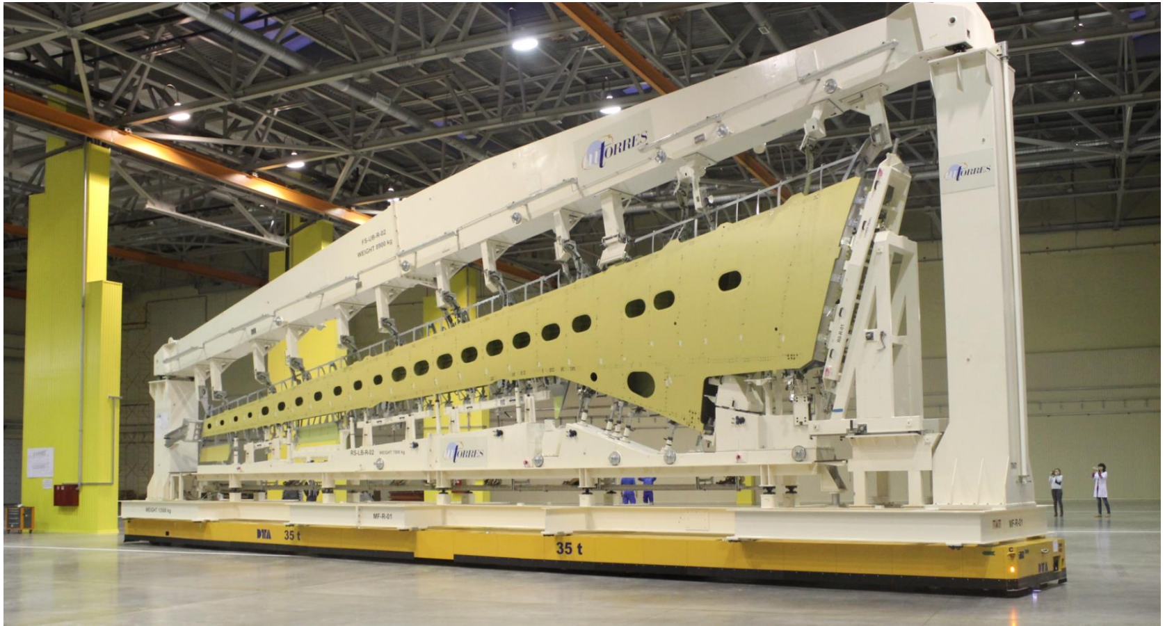
Final assembly line for the Russian MS21 wings installed in Aerocomposite (Ulyanovsk, Russia)
