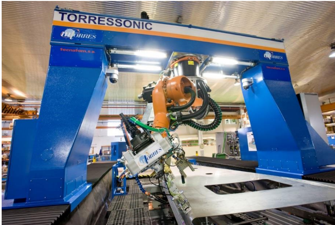
Ultrasonic inspection machine installed at Spirit Kinston ( USA) for the A-350 program
