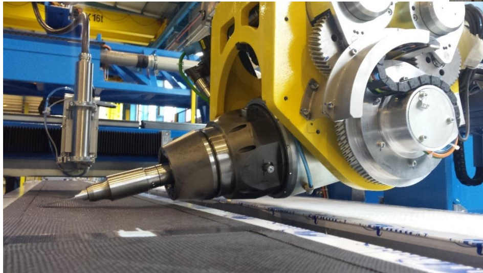
6-Axes Machine for ultrasonic cutting composite components
