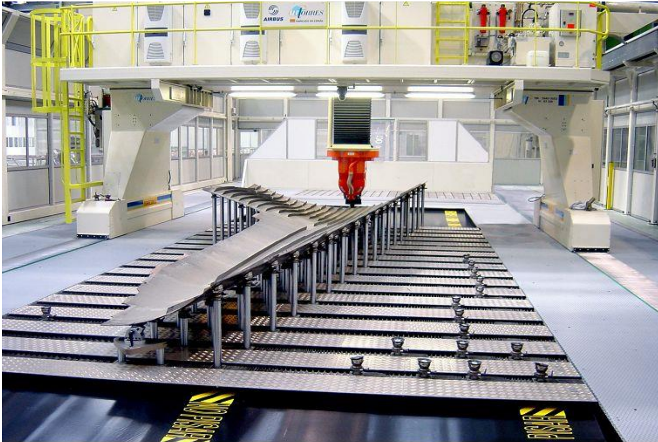
Torresmill and Torrestool machines for high speed milling and drilling of aircraft Carbon Fiber structural components for the A380 program installed in Airbus Illescas plant (Spain)
