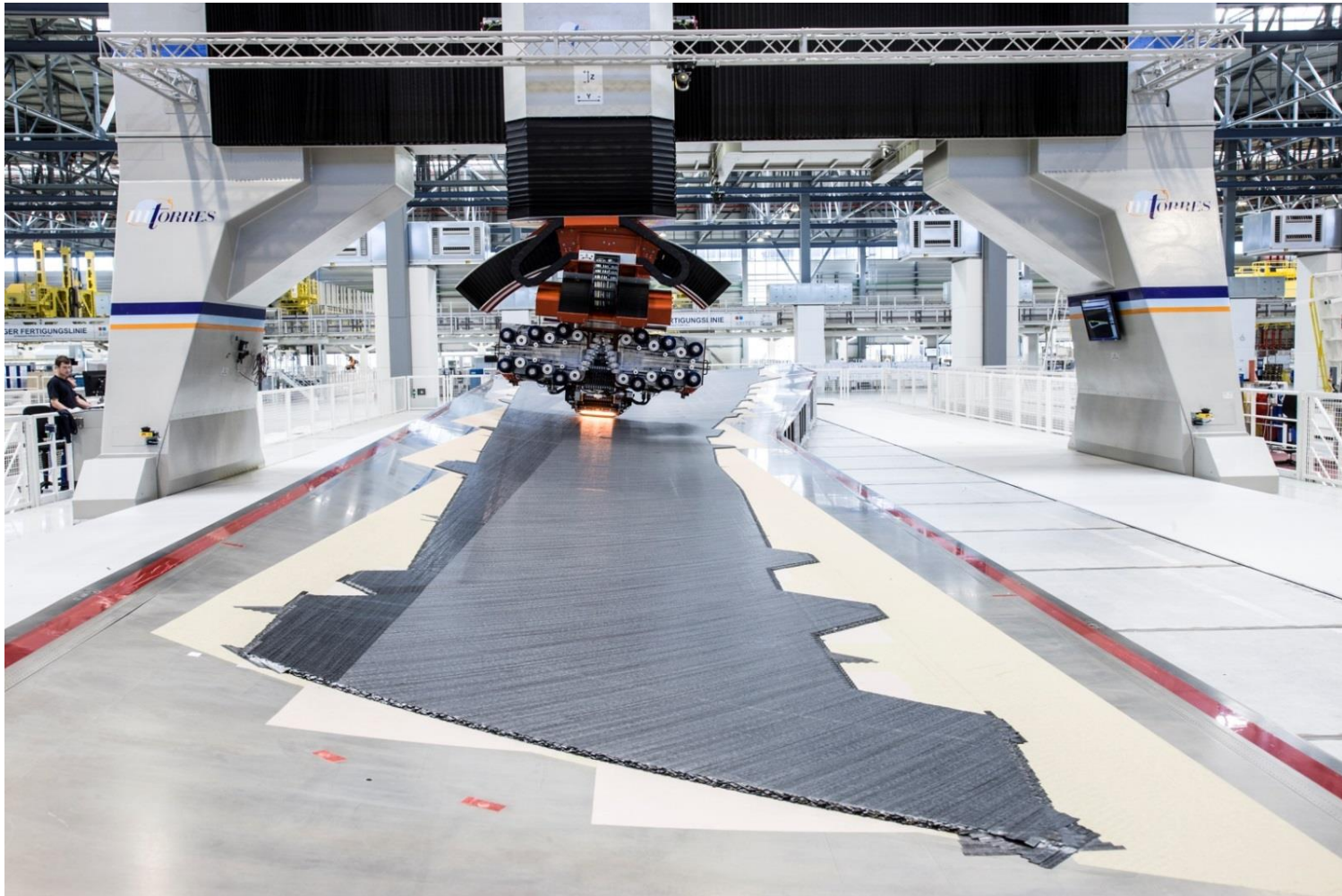
Hybrid ATL /AFP machine for A350XWB wings skins fabrication in Airbus Stade plant (Germany)
