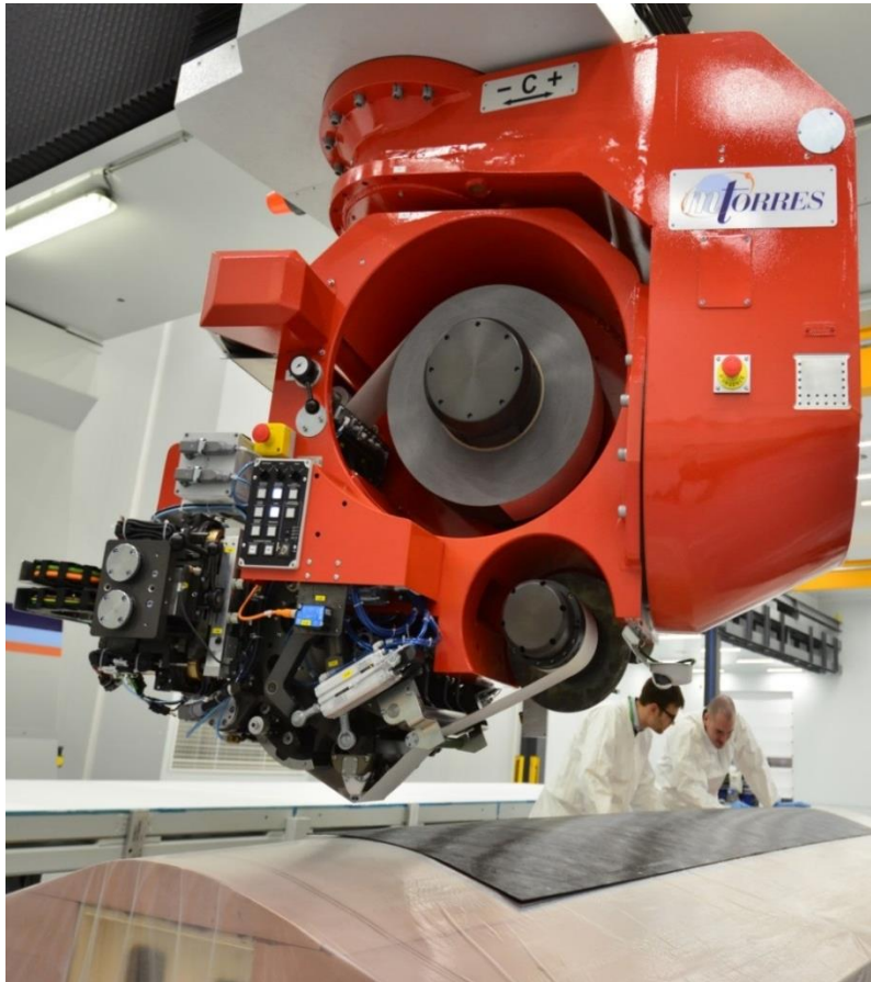
Automatic Tape Laying machine, Torreslayup, for the Embraer programs E175 and E190 installed in Sonaca (Belgium)
