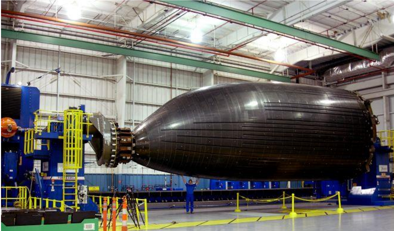
Milling and drilling Machine for fuselages of BOEING 787 program. SPIRIT AEROSYSTEMS (USA)
