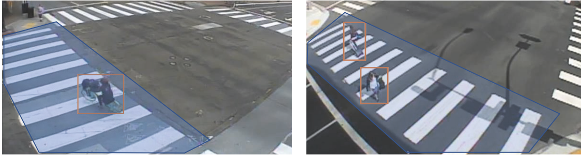
FIGURE 3: Pedestrians (right) and a bicyclist (left) detected while crossing an intersection within the region of interest.
