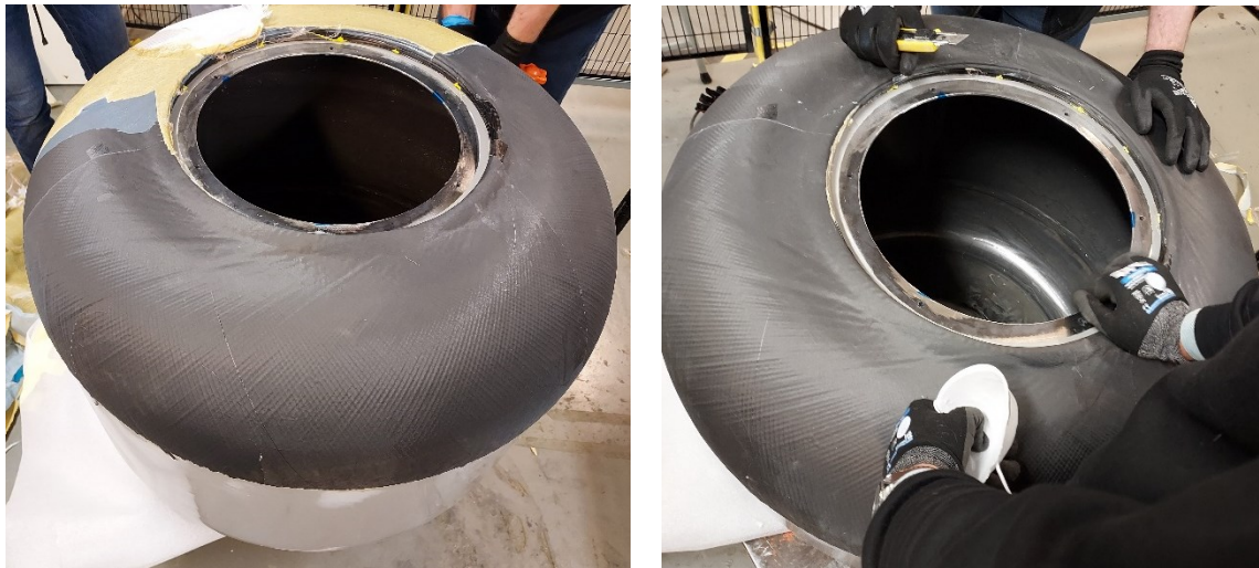
Figure 41 – Mold out of the oven and removing vacuum tools
