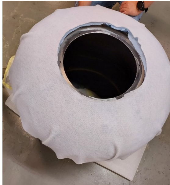
Figure 37 – Application of surface breather fabric
