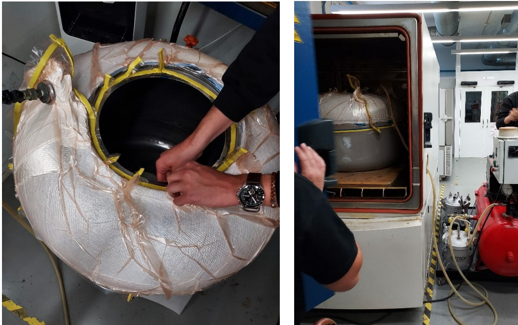
Figure 39 – Applying vacuum and inserting the mould into the oven
