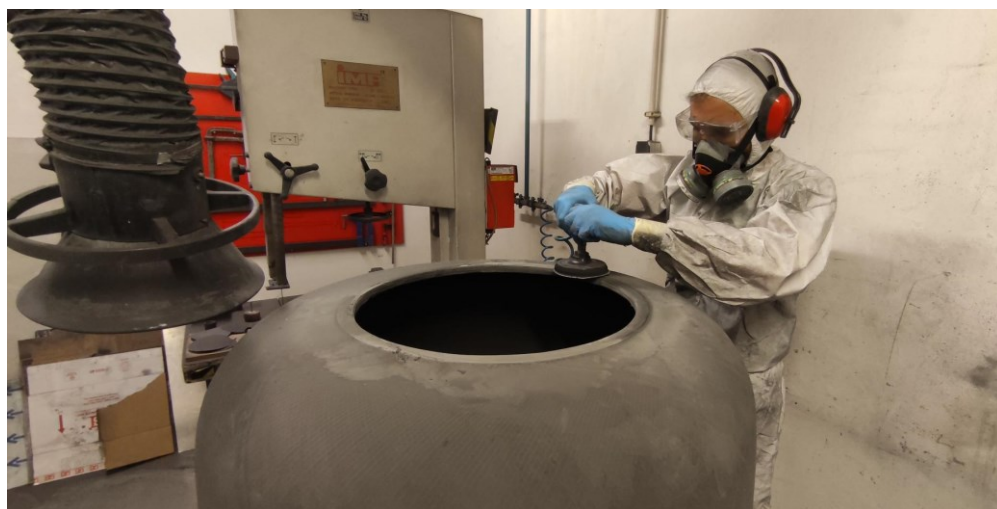
Figure 43 – Sanding of the ends with overthickness
