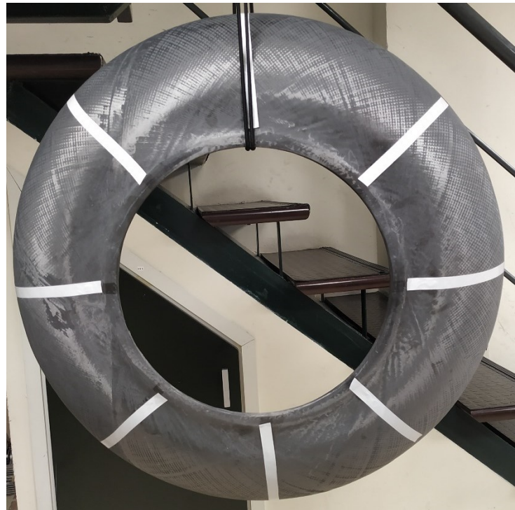
Figure 50 – Photography of Tidal Housing Demonstrator tested in this study
