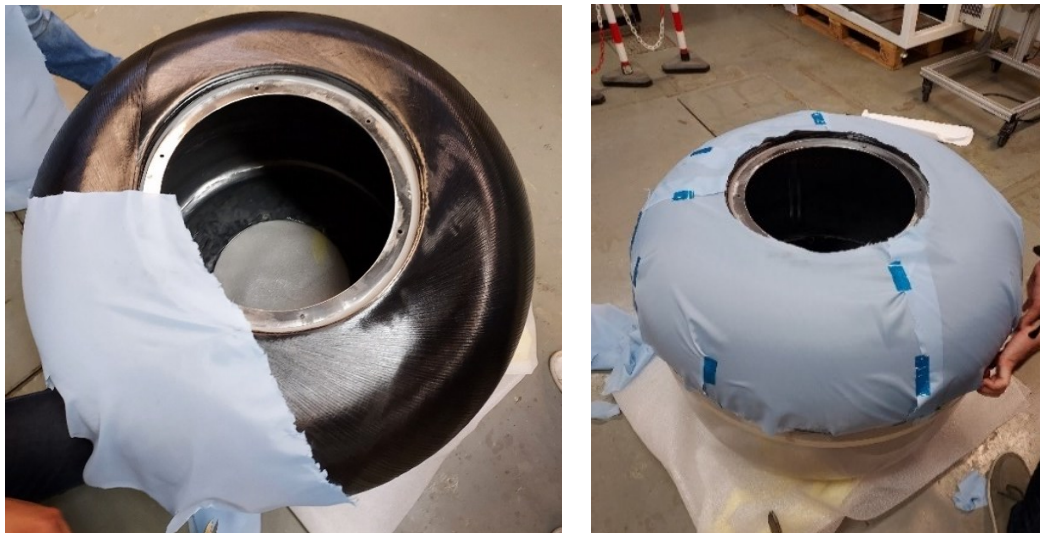
Figure 36 – Application of release fabric
