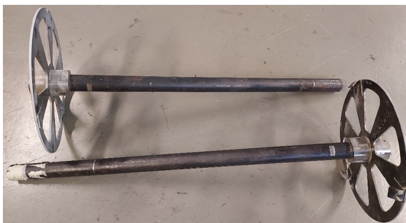
Figure 23 – Shaft and rims for connection between mandrel and robot supports
