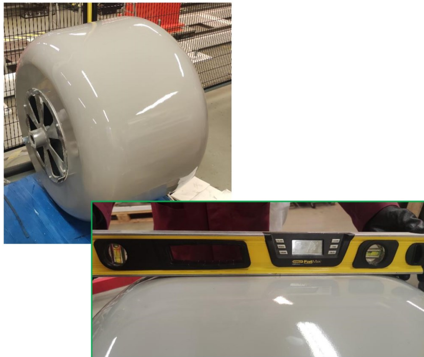
Figure 22 – Good draft angle after correction
