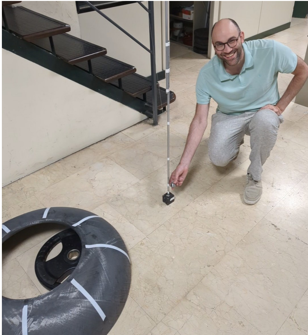
Figure 55 – Photography of tests used to evaluate the capabilities of a SHM system for the detection of impacts at low velocity impact energy levels
