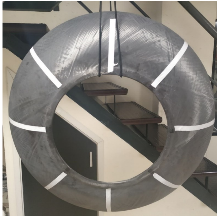
Figure 51 – Description of the vibration test used to obtain the modal parameters of the Tidal Housing. The white bands show the position of the accelerometers during the test.
