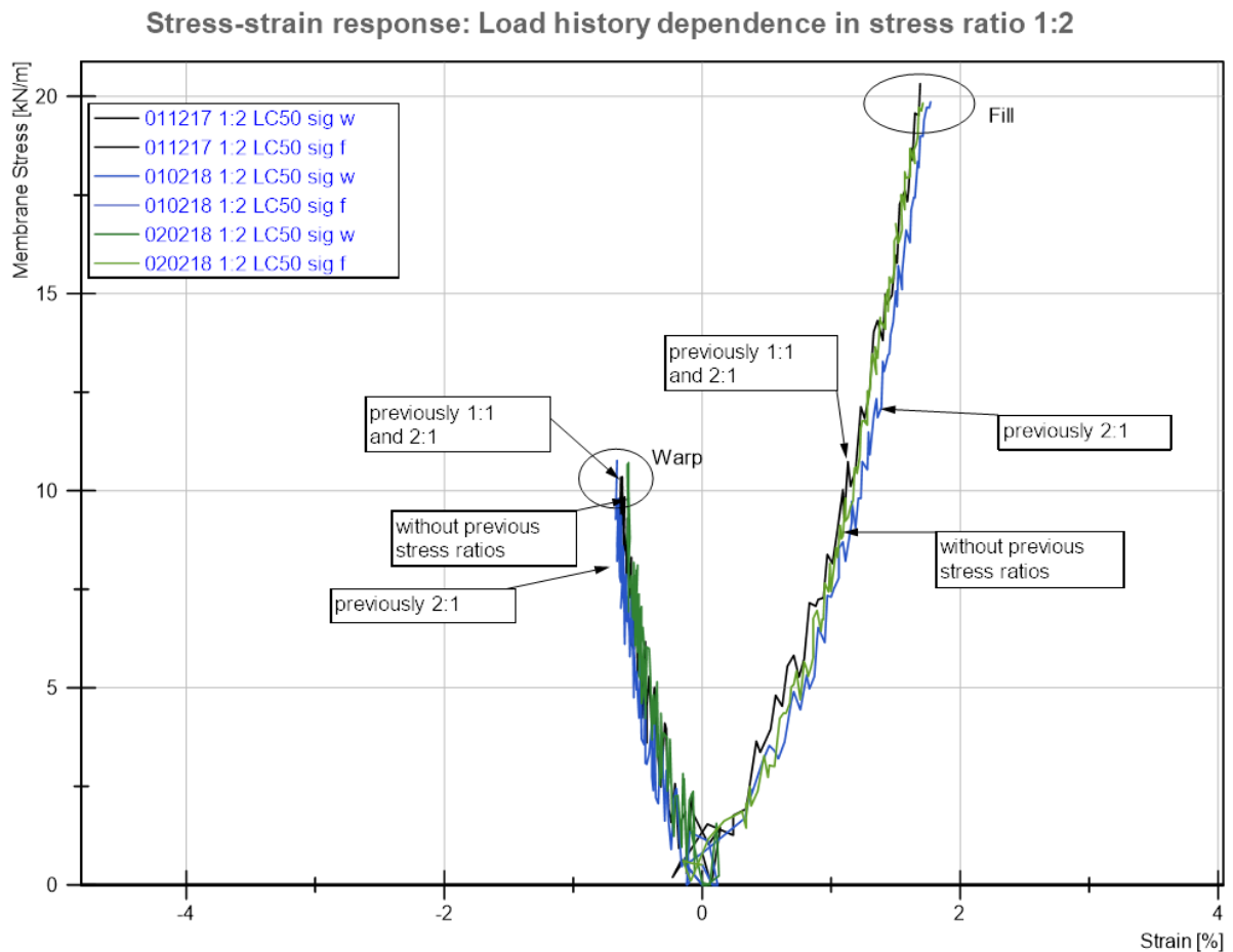
Figure 5: Stress-strain response in stress ratio 1:2
