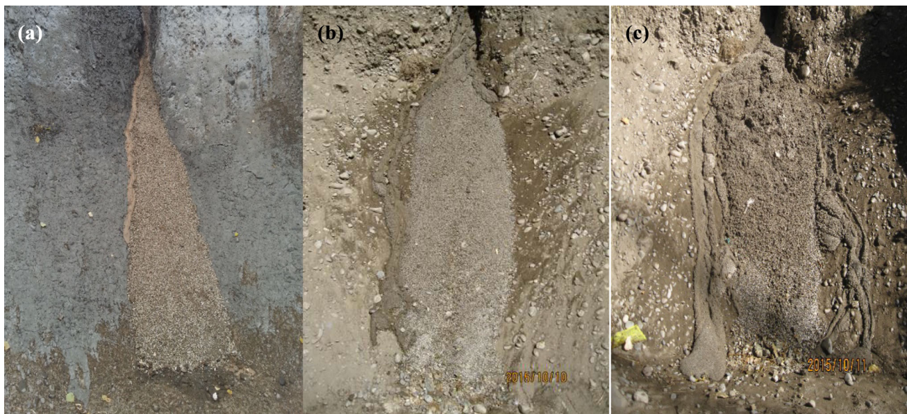
Fig. 5 Images of water–sand flow initiation under different rainfall intensity: light rainfall (a), moderate rainfall (b), and heavy rainfall (c)
