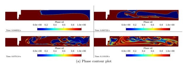
Figure 7: High-fidelity multiphase drop test case contour plots
