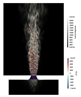
(b) Q Criterion iso-surfaces superposed on vorticity magnitude contours
