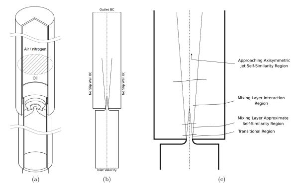
Figure 1: Shock absorber geometry and some setup details (**a**) Schematic view of the simplified shock absorber geometry; (**b**) The computational domain with the applied boundary conditions; (**c**) Axisymmetric shear layer development regions, following Bradshaw et al. [1].
