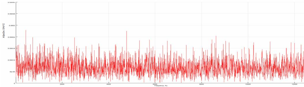
**Figure 8** Sample of vibration sensor spectrum noise density
