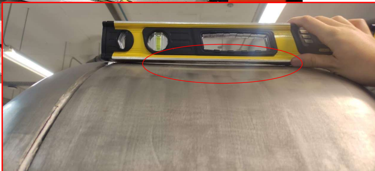
Negative draft angle due to sinking/warping
