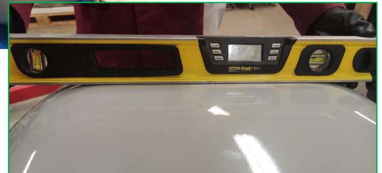
Good draft angle after correction
