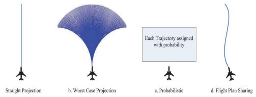
Fig. 5. Projection types of encounter's state vector
