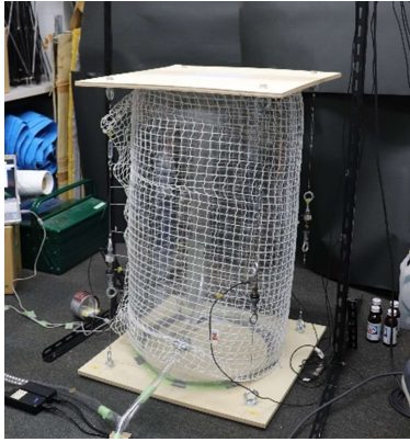
Fig.1.1: An example of air column, which is used by loading test
