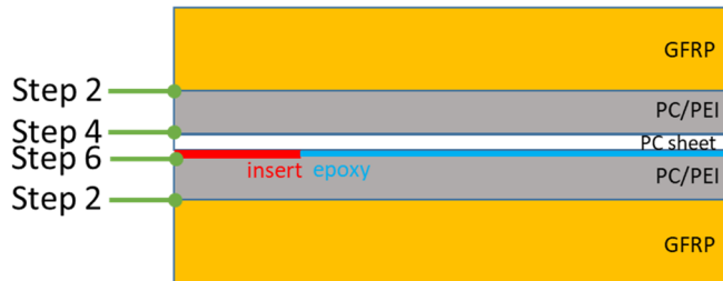
Figure 13. Bonding steps for AM specimens.
