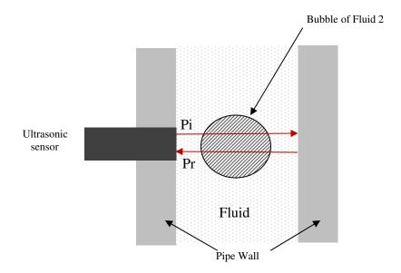
Fig. 14. Ultrasonic waves reflections with the presence of large bubbles.
