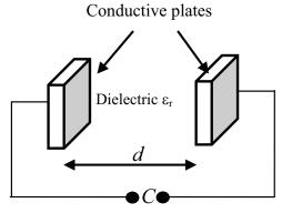
Fig. 4. Simple configuration of a capacitance.
