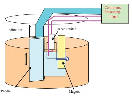
Fig. 9. Block diagram of the vibrating Switch for interface measurement
