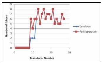
Fig. 17. Detecting the emulsion layer using the number of echoes.
