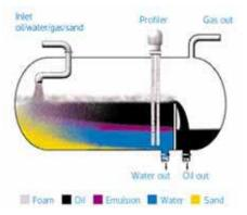
Fig. 7. The Nucleonic Tracerco's level measurement system ([18,19]).
