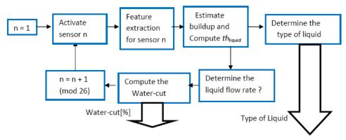
Fig. 21. Bloc diagram of the pattern recognition algorithm.
