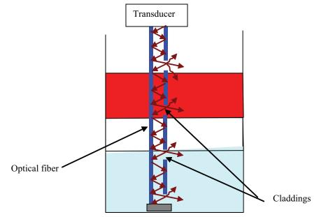
Fig. 10. Principle of multi-level measurements using optical fiber.
