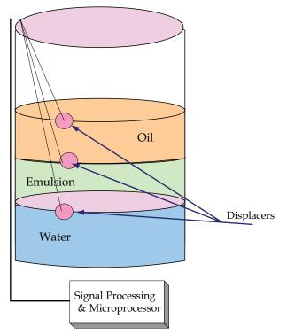
Fig. 8. Displacers floating at top of each liquid.
