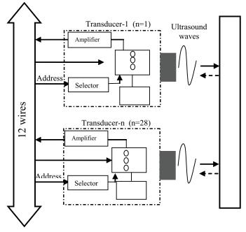
Fig. 24. Electronic design: Transducer-Transducer connections.
