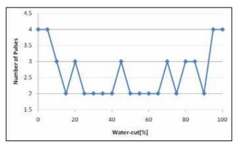
Fig. 18. Number of pulses versus water-cut.
