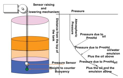
Fig. 3. Varying pressure as sensor level is changed.
