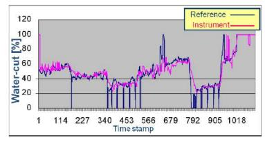
Fig. 26. Plot comparing the measured water-cut versus the reference.
