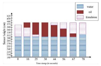
Fig. 29. Dynamic tracking of the emulsion layer.
