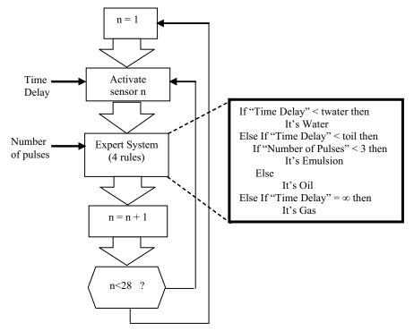
Fig. 22. Flow chart of the pattern recognition algorithm
