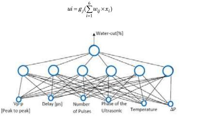
Fig. 23. Neural Network algorithm for water-cut determination
