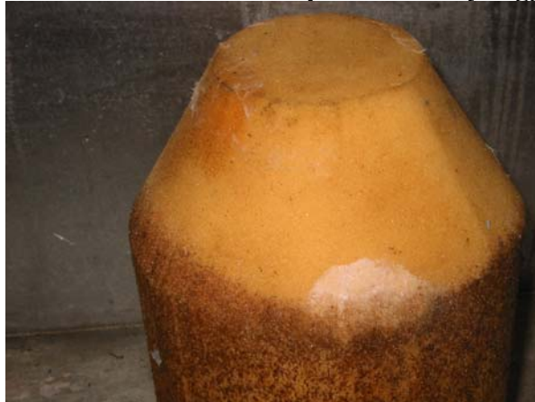
Photo 22: Soft Sealant Lump Removed by Pigging
