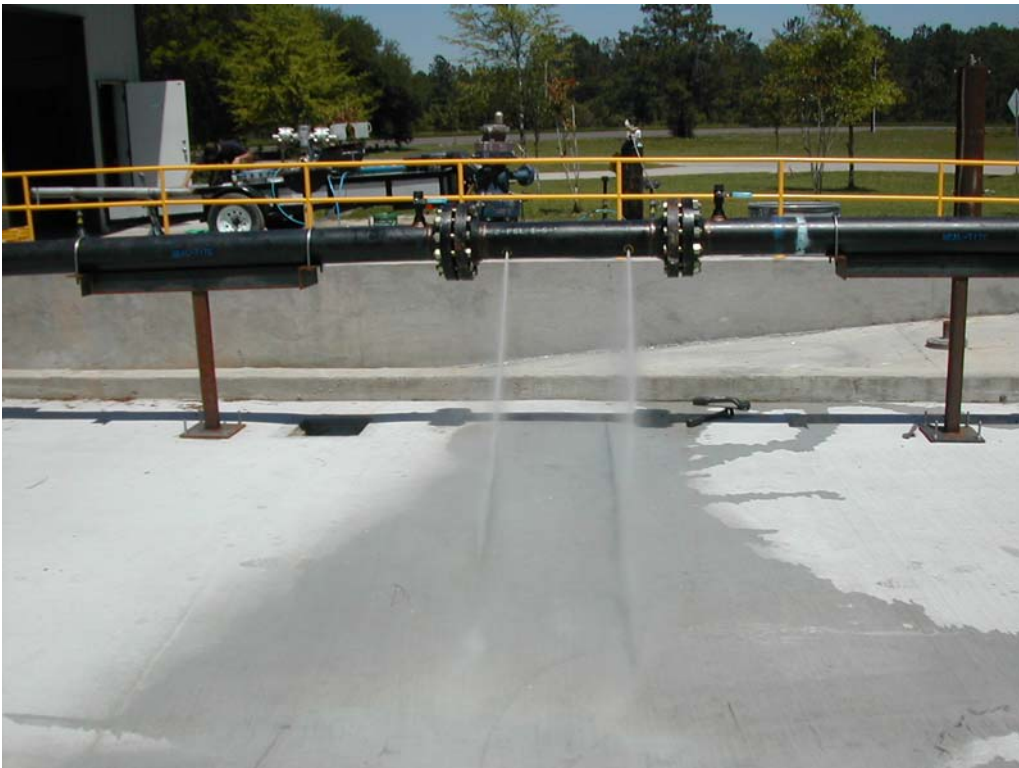
Photo 11: Pinhole Leak Rate Testing
