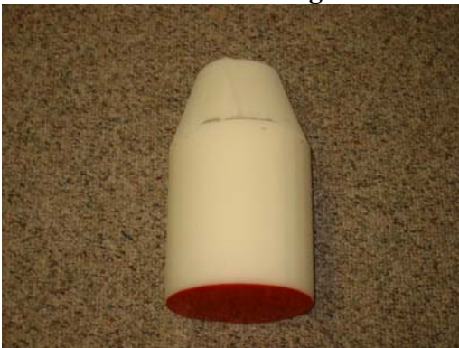
Photo 13 2 lbm/ft 3 Yellow Swab Pig with Nose
