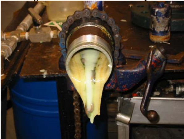
Photo 33: Draining Uncured Sealant from Cylinder
