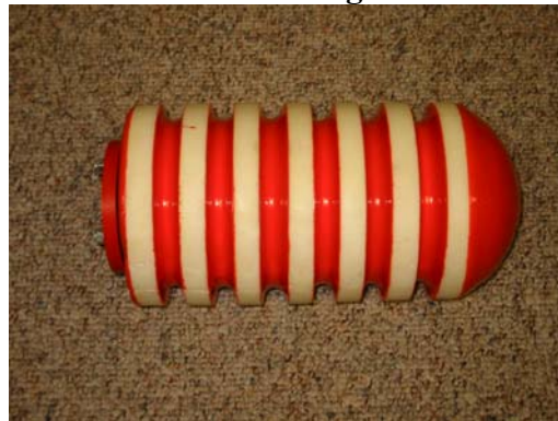
Photo 14 5 lbm/ft 3 Foam Disc Pig with Nose
