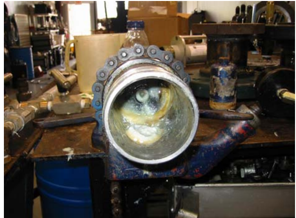
Photo 34: Sealant Across Defect
