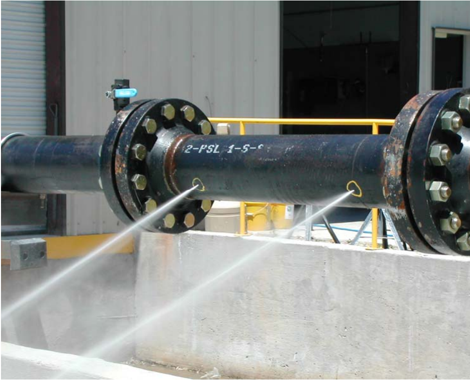
Photo 10: Pinhole Leak Rate Testing
