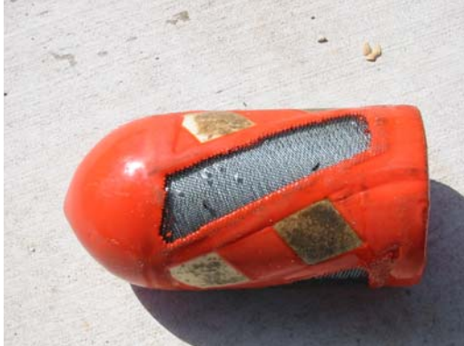
Photo 15: 5 lbm/ft 3 Foam Crisscross Wire Brush Pig with Nose
