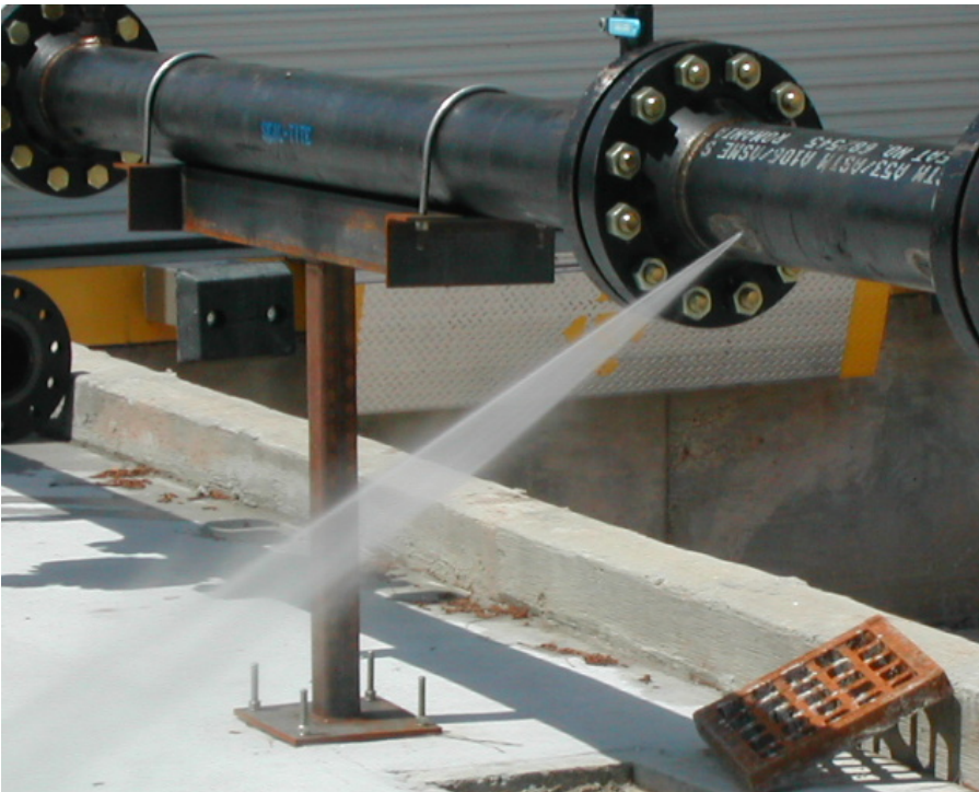
Photo 7: External Corrosion Leak Rate Testing
