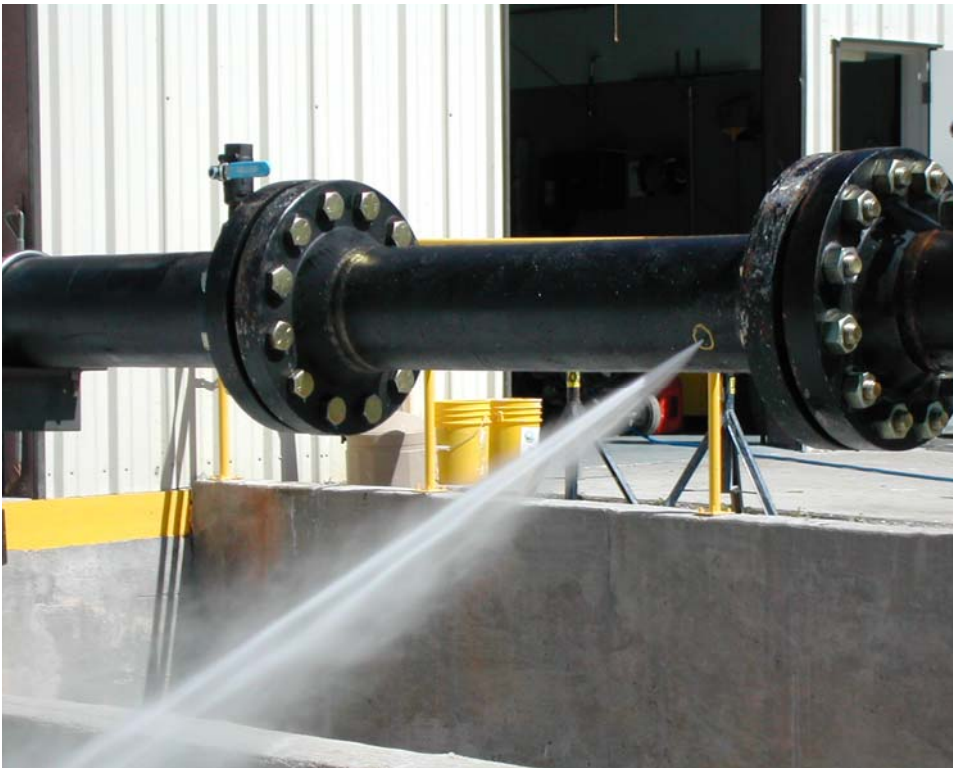
Photo 9: Internal Corrosion Leak Rate Testing
