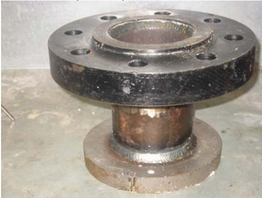
Photo 23: 114.3 mm (4-1/2") Test Fixture
