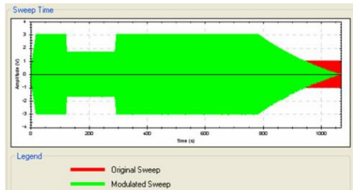
Fig. 8 : Example of amplitude-modulated excitation signal
