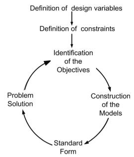
Fig. 2 Phases of MDO design and optimization method
