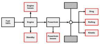
Fig. 4 Losses in a ground vehicle
