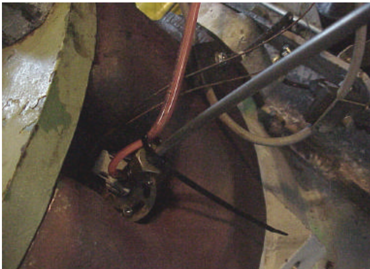
Closeup of Delphi pilot fuel injector installed in head
