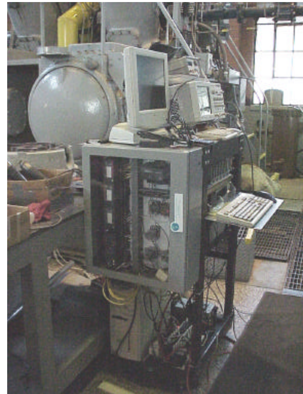
Micropilot control system for engine operation
