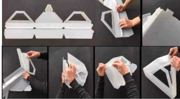
Figure 5. Cassette assembly by folding.
