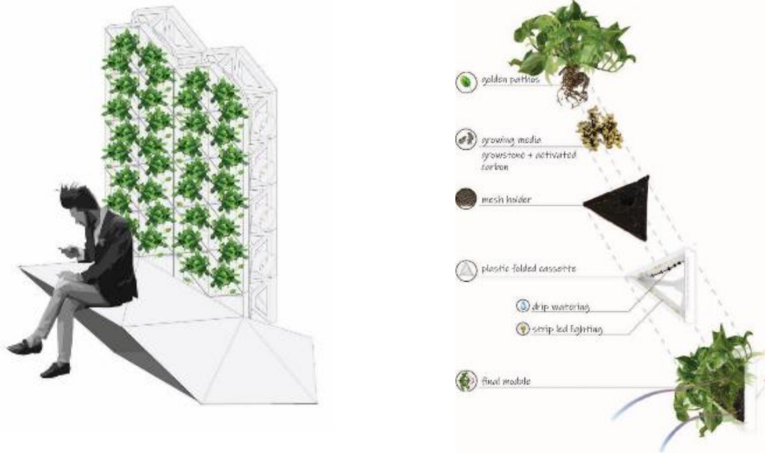
Figure 2. a. The double-sided prototype of plant-base air filtering system; b. Components of plant-based air filtering system.
