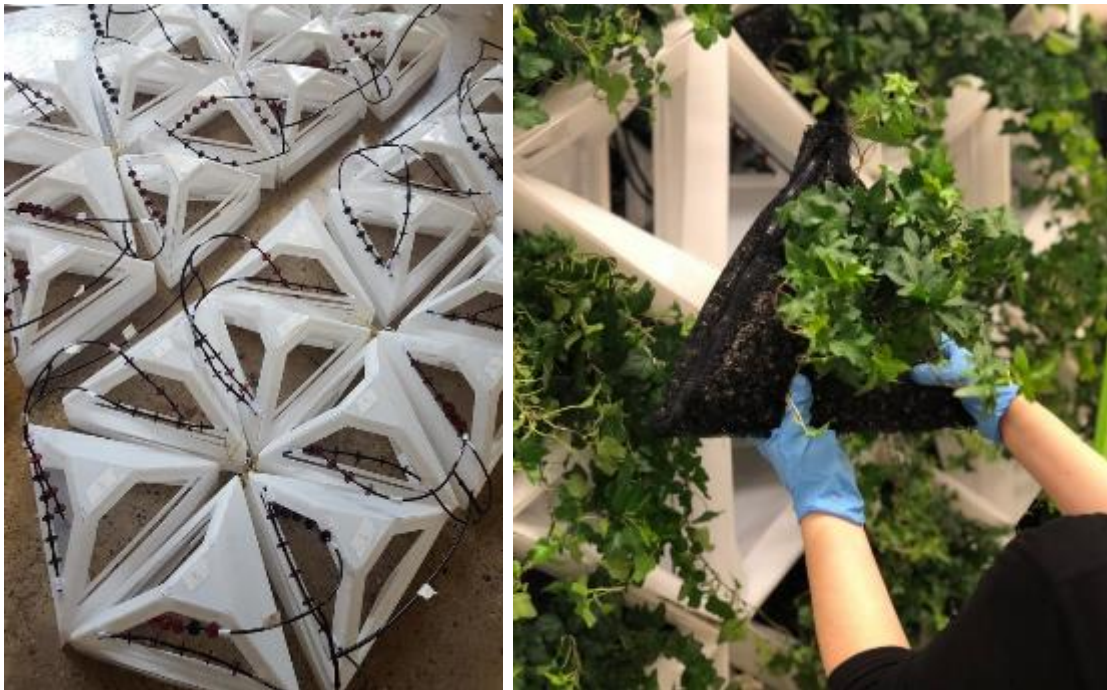
Figure 3. a. Folded cassettes and dripper attachments; b. 3d mesh holding growing media and plants.
