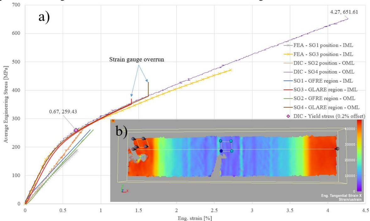
**Figure 7: a) Stress-strain curves for: FEA predictions, DIC and strain gauge measurements; at GLARE and GFRE regions of test specimen MST-C-01; b) Longitudinal engineering strain field at maximum load.**
