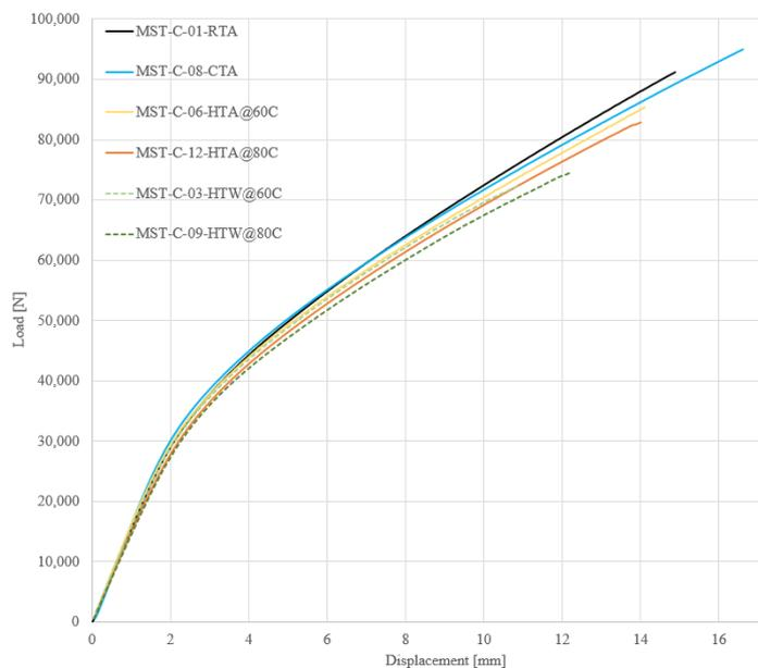
**Figure 6: Load-displacement curves of C-configuration structural element specimens tested at different ambient conditions.**
