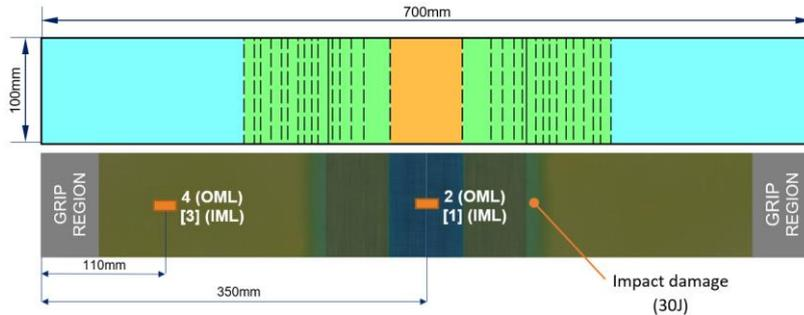
**Figure 5: Structural element test specimen - OML view: drawing showing material regions (top) and photo with specified strain gauge, grip and impact locations (bottom).**
