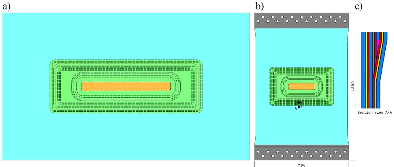
**Figure 1: Panel drawings: a) demonstrator panel; b) test panel; four different regions and corresponding materials are color coded: GLARE 3 in light blue, S2/GFRE in orange, GLARE 3 – GFRE transition in green and aluminium bonded tabs in gray c) section view A-A: ply drop detail.**
