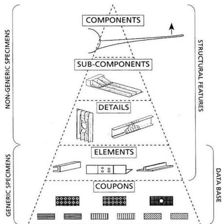
Figure 4: Aerostructures testing pyramid.
