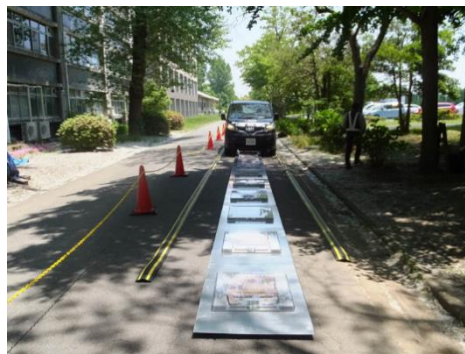
Figure 10. Photograph of the dynamic WPT system in the real-car test.
