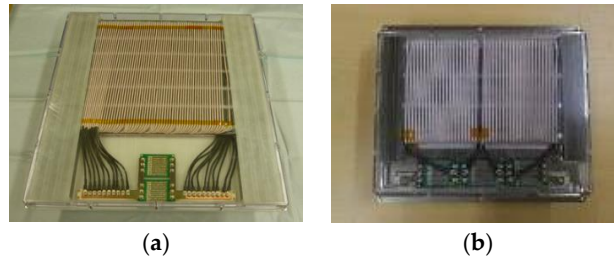
Figure 2. Photographs of the WPT coils tested in this paper. (a) Ground-side coil, (b) vehicle-side coil.
