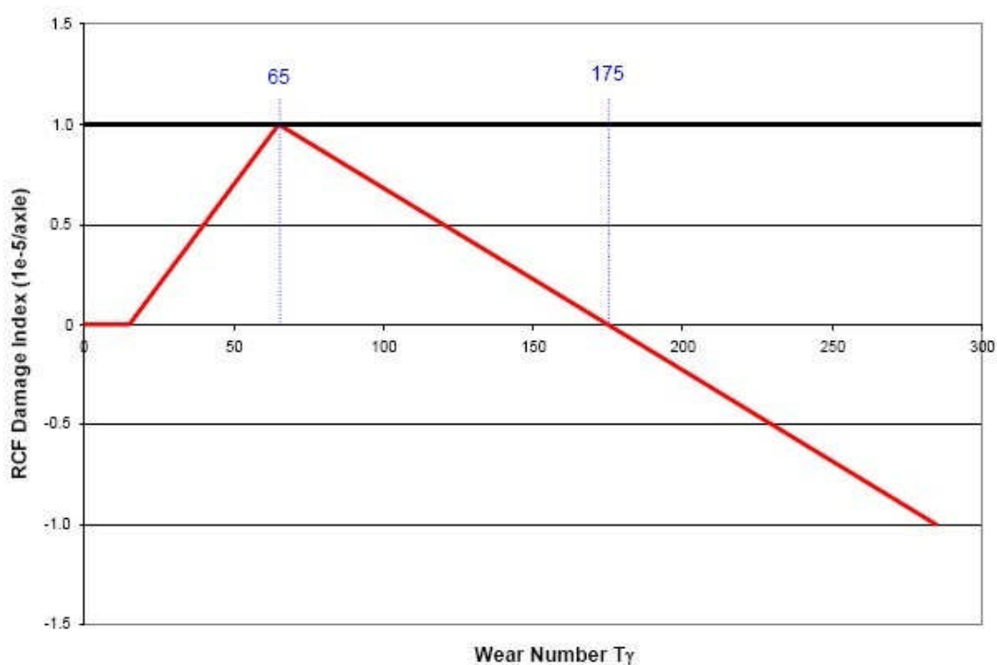
Figure 1: Relationship between wear number ( T\gamma ) and RCF damage index
