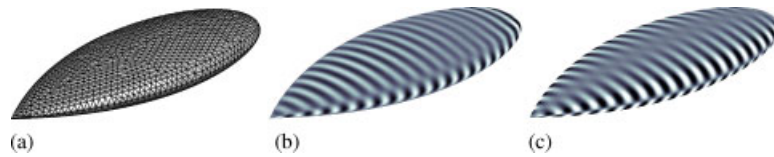
Figure 32. Scattering by a PEC NASA almond of characteristic length 21\lambda : surface mesh on the almond and two components of the scattered field for a NEFEM solution with p=3 : (a) surface mesh; (b) E_3 ; and (c) H_3 .
