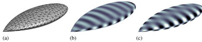
Figure 30. Scattering by a PEC NASA almond of characteristic length 8\lambda : surface mesh and two components of the scattered field for a NEFEM solution with p=5 : (a) surface mesh; (b) E_3 ; and (c) H_3 .
