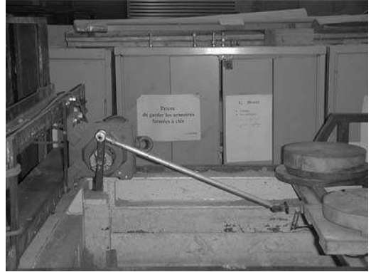
Figure 2. Loading system for displacement controlled tests.
