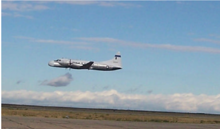
Figure 6. Space Systems’ ANGEL System test aircraft – General Dynamics Convair 580 (NC-131H) turboprop landing at the Natrona County International Airport, Casper, Wyoming
