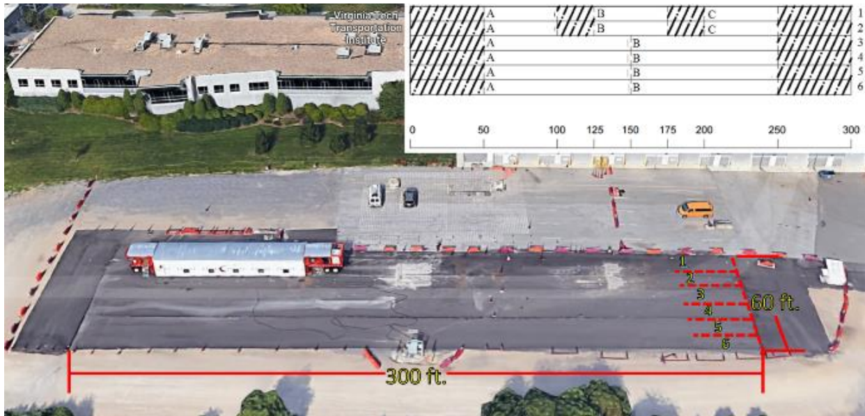
Figure 4: Dimensions of pavement test sections.
