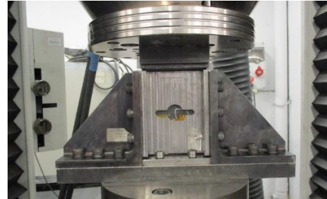
Figure 4. CAI test set-up with anti-buckling device.
