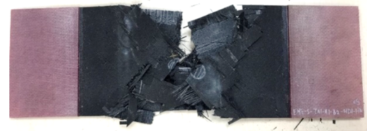
Figure 13. M4-EME TAI specimen after testing under HW conditions.
