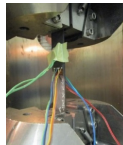
Figure 1. Tension test set-up (HW conditions).
