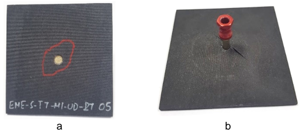
Figure 11. M4-EME Pull-through specimen after testing under RT conditions.
