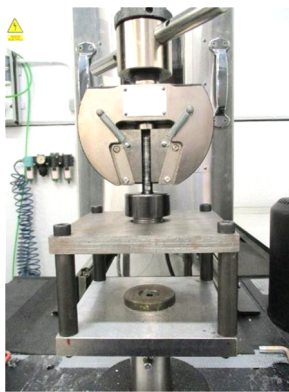
Figure 3. Pull-through resistance test set-up (RT conditions).
