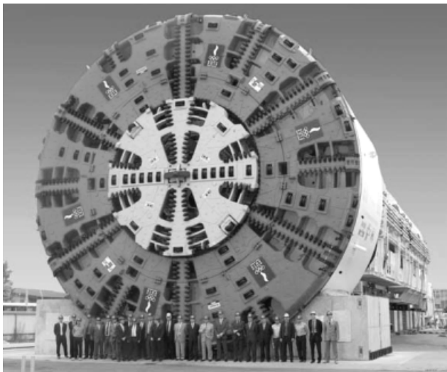
Fig. 75. Herrenknecht EPB machine, 15 m in diameter, for urban motorway tunnel in Madrid
