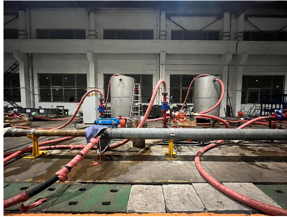
Figure 5: Layout of hydraulic lift type dual-gradient drilling indoor physical simulation experiment system
