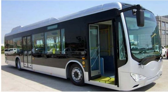
Figure 13. BYD eBUS-12 electric bus.
