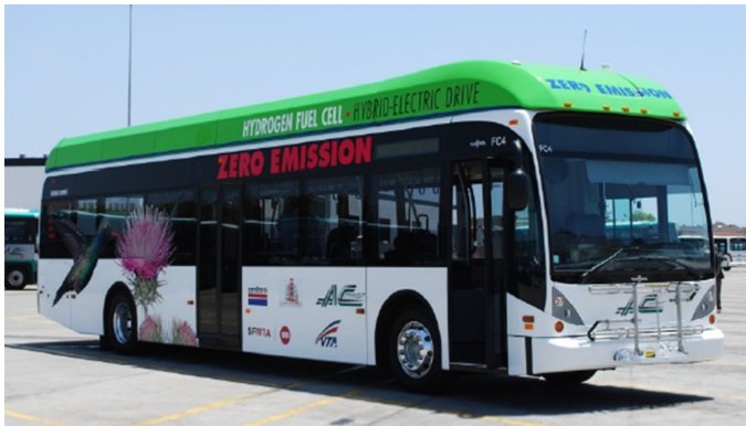
Figure 11. The new Van Hool fuel cell bus.
