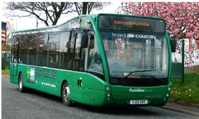
Figure 16. Optare's battery-powered Versa.
