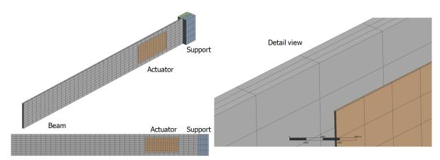
Figure 6: Mesh of the finite element model
