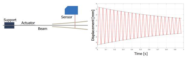
**Figure 4**: Free vibration test:  $1^{st}$  bending vibration mode (black dashed line - damping envelope: damping ratio  $\zeta = 0.6 \%$ )
