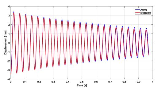
Figure 8: Comparison between free vibration of measured and simulated system
