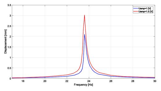
Figure 5: Forced vibration test: displacement amplitude-frequency characteristics
