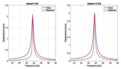
Figure 9: Comparison between frequency response of measured and simulated system
