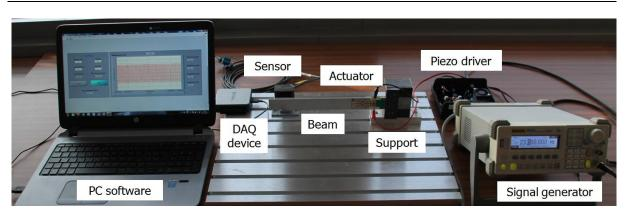
Figure 3: The real experimental setup
