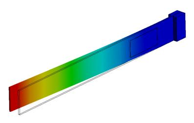
Figure 7: Modal analysis: beam's 1<sup>st</sup> vibration mode at 23.64 Hz
