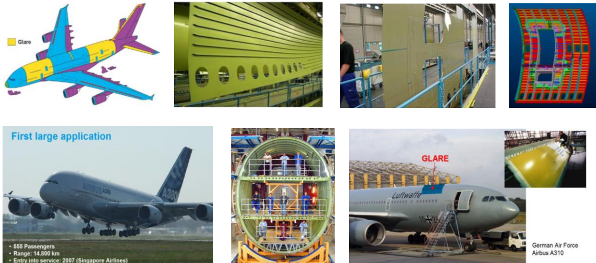
Figure 3: FML Glare application examples (clockwise from top left): Glare FML panels on A380, FML panel with stringers and window cut-outs, FML door panel, door panel design, developmental Glare test panel flown on A310, A380 fuselage cross section (Megaliner Barrel test), A380 take-off
