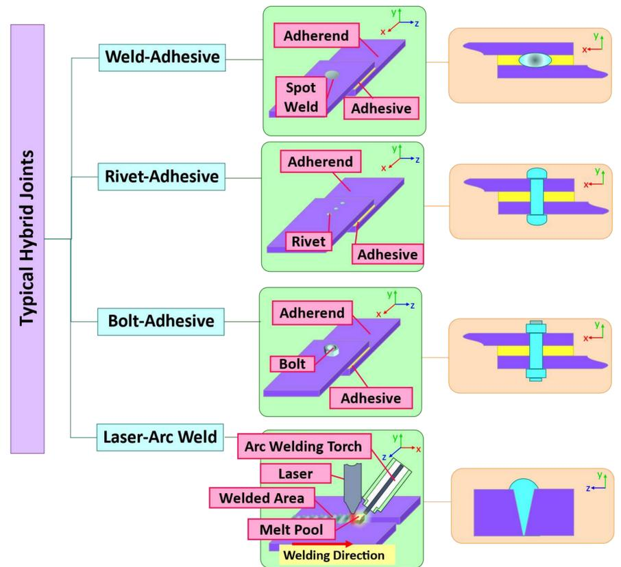
Figure 3 – Typical hybrid joints in the marine industry
