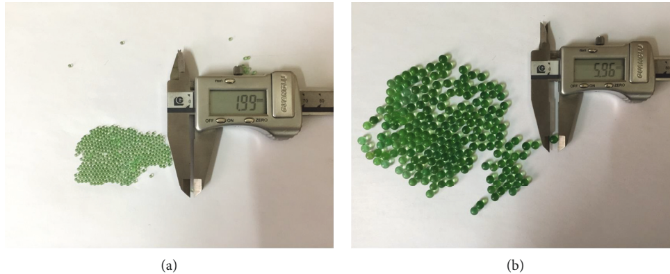
FIGURE 8: Green glass beads used in the experiment: (a) \Phi 2 mm diameter, and (b) \Phi 6 mm diameter.
