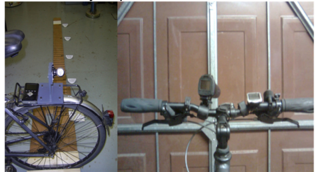
Fig. 1. Instrumented Bicycle, AT1 Camera/ Receiver, Mount, Cycle Stand and Graduated Board and ATC 5K Bar Mounted Camera.
