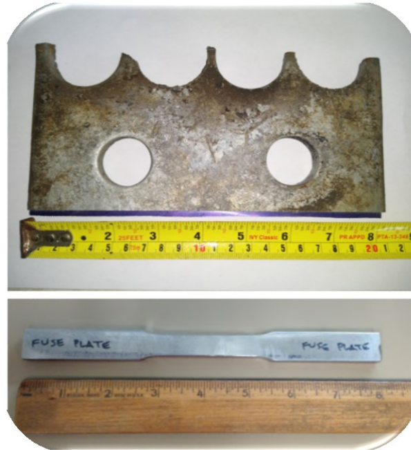
Figure 6: Actual fuse plate that failed and the specimen machined from the bottom of the plate.
