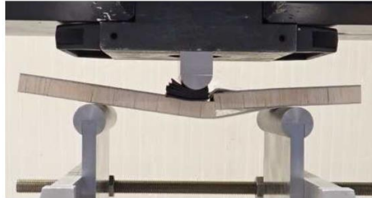
Sandwich lay-up (polyester GFRP + balsa wood)
