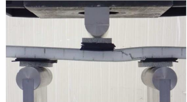
Sandwich lay-up (epoxy GFRP + PET foam)
