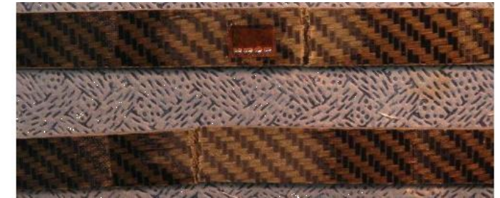
Tensile test on woven flax/basalt monolithic coupons
