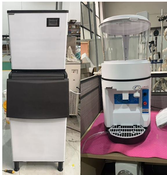
Figure 2: Ice making and ice crushing equipment
