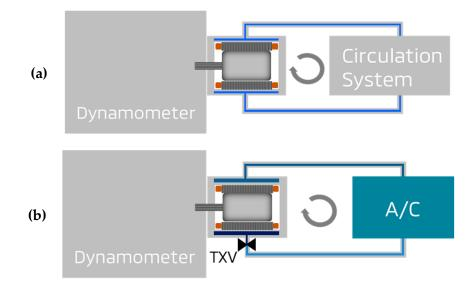
Figure 4. Experimental setup: (a) Water cooling; (b) refrigerant cooling.
