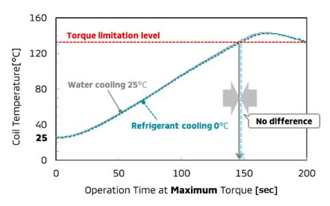
Figure 9. Coil temperature vs operation time at maximum torque.
