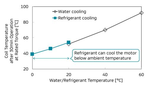
**Figure 6.** Coil temperature after 30 min operation at rated torque vs water temperature or refrigerant temperature.
