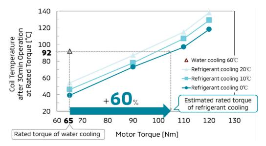
Figure 8. Coil temperature after 30 min operation vs motor torque.
