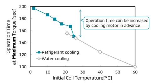
Figure 11. Operation time at maximum torque vs initial coil temperature.
