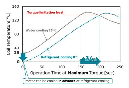
**Figure 10.** Coil temperature vs operation time at the maximum torque in case that refrigerant cooling cooled the motor in advance.
