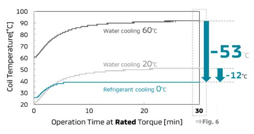
Figure 5. Operation time at rated torque vs coil temperature.
