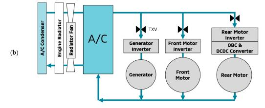
**Figure 2.** (a) Current cooling system of PHEV; (b) one example of ideal cooling systems using refrigerant cooling.
