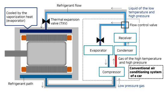
Figure 1. Proposed refrigerant cooling system.
