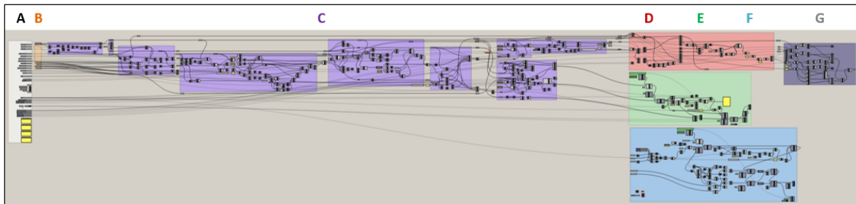
Figure 3: Tensys GH script for parametric generation of 3D surface model and the initial topology for the HOWL project. A – Control panel for adjustment of model parameters, preview and export of the inTENS topology; B – Imported model of the site; C – Generation of the reference curves; D – Generation of lofted surface for visualisations; E – inTENS topology generation using Tensys Rhino Tools Plugin components; F – Generation of inTENS patterning model topology from an imported analysis shape; G – Generation of seam lines for visualisations.
