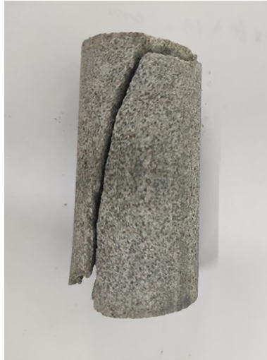
Figure 4: Triaxial shear test phenomenon of sand hydrate sediment samples [22]
