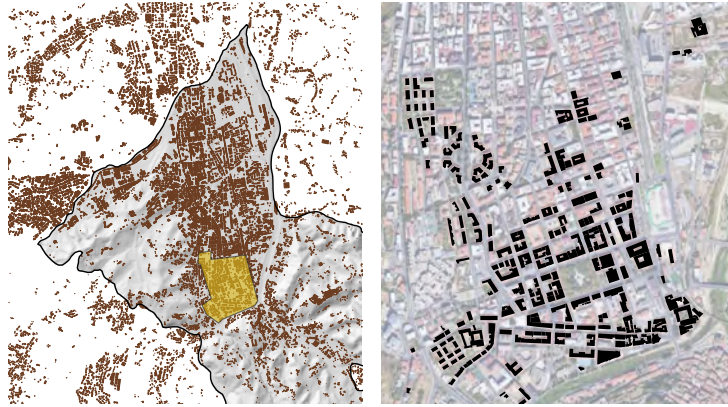
Figure 1: Location of the studied district on Cosenza urban area (left-hand side) and, in black, the masonry structures considered in the seismic vulnerability assessment (right-hand side).
