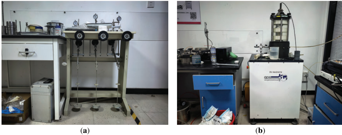
Figure 8: Test equipment: (a) Triple-cell consolidation apparatus (Suzhou Top-Test Instrument Co., Ltd., Suzhou, China); (b) Triaxial apparatus (GDS Instruments, Global Digital Systems Ltd., Hampshire, UK)
